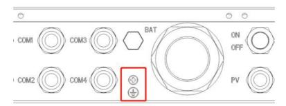
**Note:** As far as possible, the ground cable should be much thicker as possible (the sectional area of wire should not be less than 4mm<sup>2</sup>), and the grounding point should be kept close to the Inverter as possible. The ground wire shall be shorter as possible.
