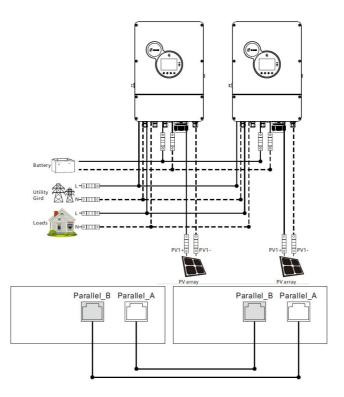
b) Three all-in-one solar charger inverters of the system connected in parallel:
