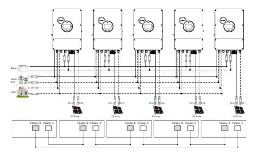
e) Six all-in-one solar charger inverters of the system connected in parallel:
