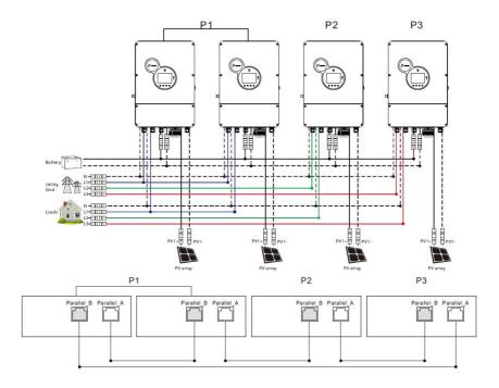
Five all-in-one solar charger inverters of the system connected in three phase:
