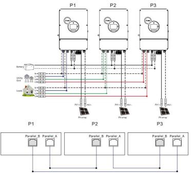
Four all-in-one solar charger inverters of the system connected in three phase: 2+1+1 system:
