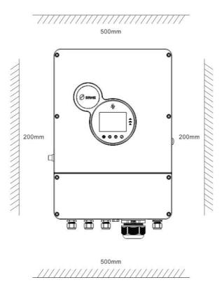
**Step 2:** Open 4 holes in the wall according to the following dimensions, and knock in expansion screws, as shown in the following figure:
