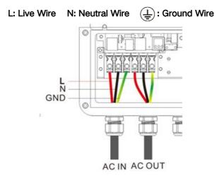
③ Connect the AC output line properly according to the cable sequence and terminal position shown in the above figure. Please connect the ground wire first, then the live wire and the neutral wire.
